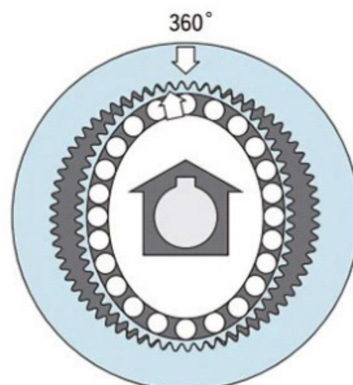
For every one full rotation clockwise (360 degrees) of the wave generator, the flexspline moves counterclockwise by two teeth relative to the circular spline because the flexspline has two fewer teeth than there are on the circular spline. In general, this movement is treated as output performing.
