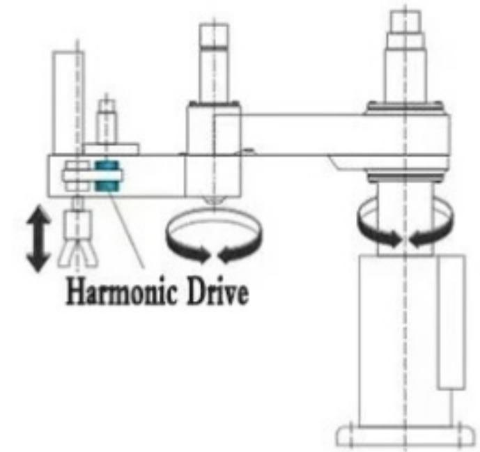
Wafer transfer robots
