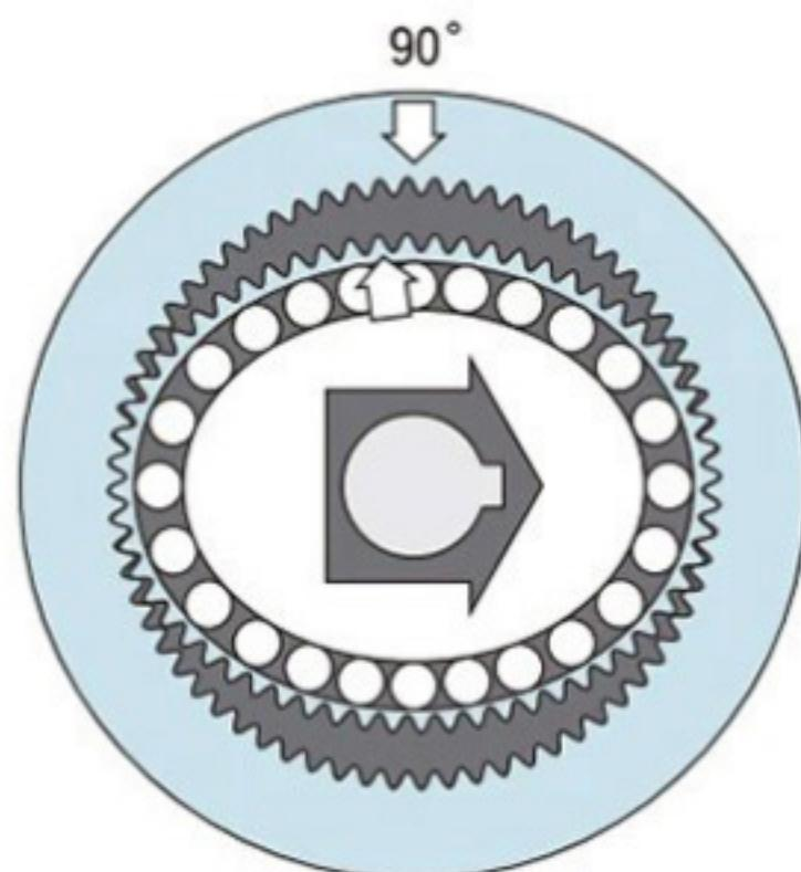
As the wave generator rotates clockwise with the circular spline fixed, the flexspline is subjected to elastic deformation and its tooth engagement position moves turning relative to the circular spline.
