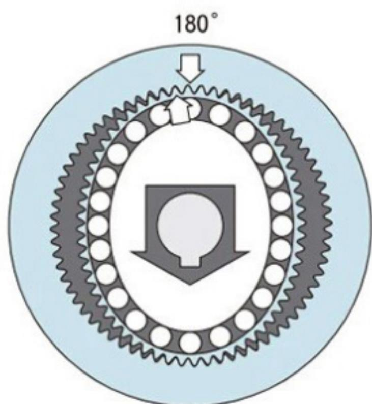
As the wave generator rotates 180 degrees clockwise, the flexspline moves counterclockwise by one tooth relative to the circular spline.
