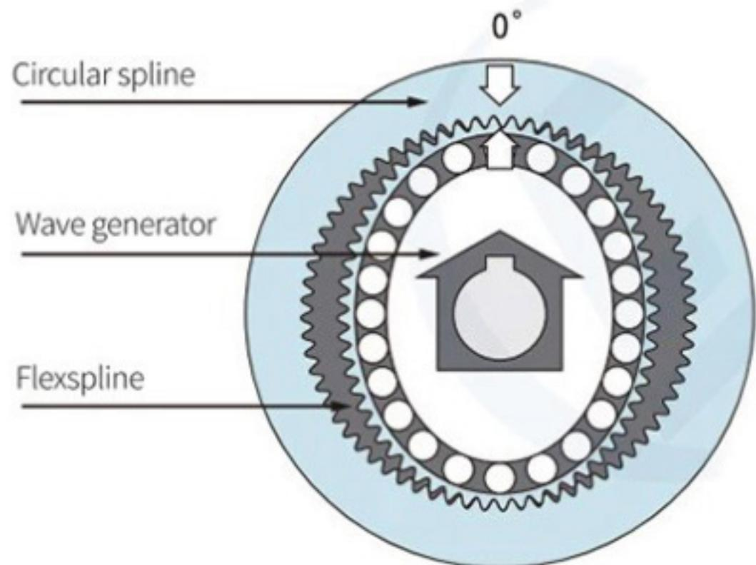
The flexspline is forced into an elliptical shape by the wave generator causing the flexspline teeth to engage with the tooth profile of the circular spline along the major axis of the ellipse, with the teeth completely disengaged across the minor axis of the ellipse.
